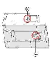
lifting the tube to remove. The tubes should be empty prior to removal The AB and EF tubes can be changed by unlocking the side latch, then
